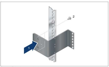
Figure 3: Fitting the support bracket
